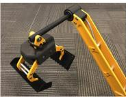
CanAssist designed the device to be very durable. Safety features ensure the gripper doesn't crush items being picked up and reduce the chance of damage to walls or floors.
